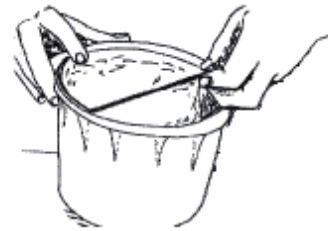
Remove o-ring in use
